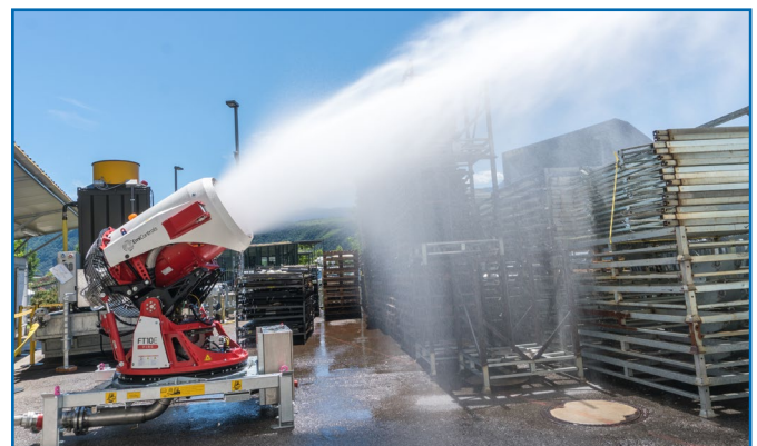
Picture 3: Spray Pattern: Fine water mist
