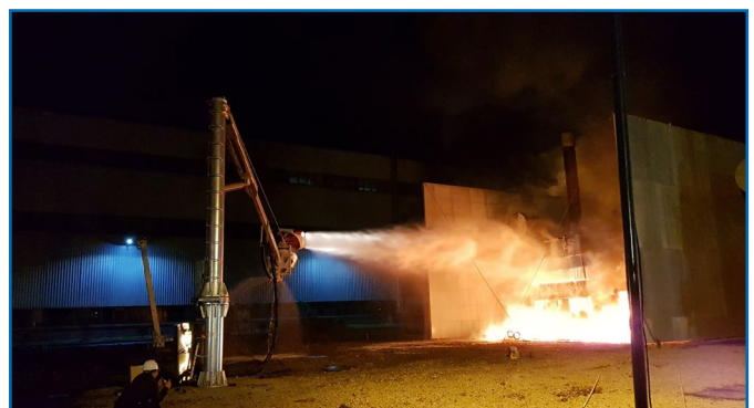
Picture 1: Water mist has a high cooling capacity with low water consumption
