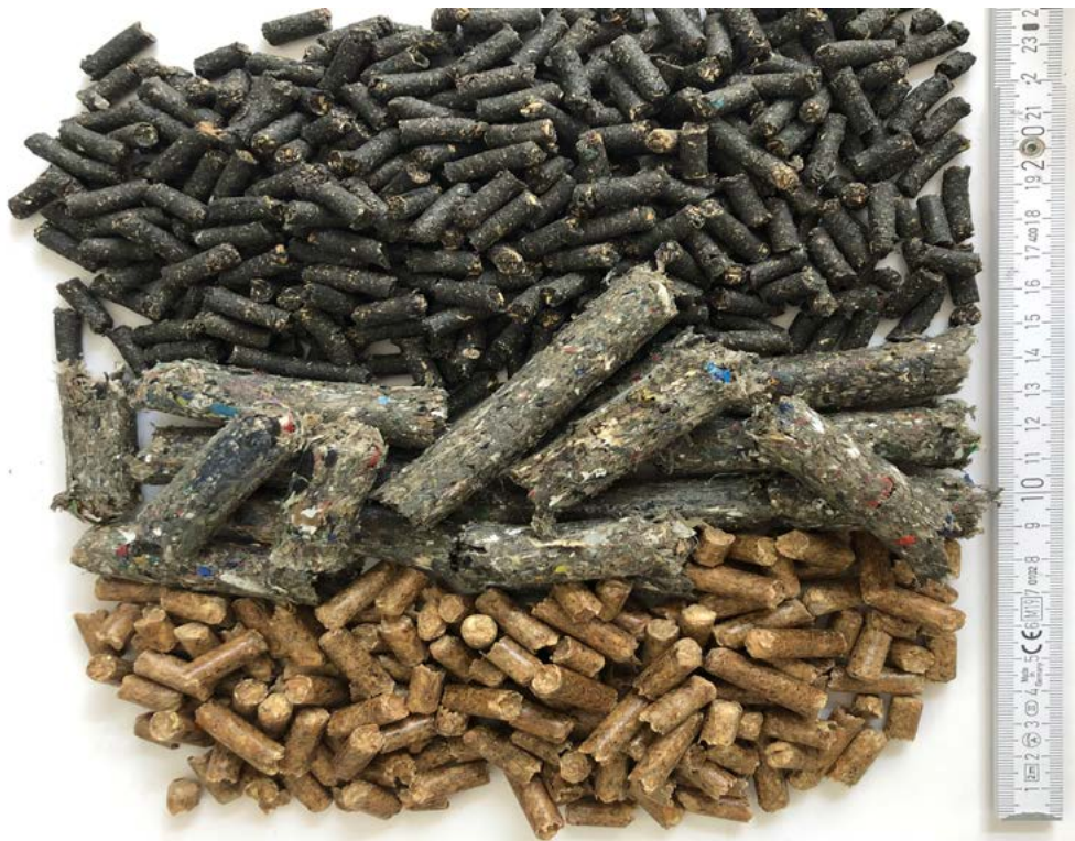
Figure 3: Pellets – 6mm RDF/wood mixture (top), 16mm RDF (middle), 6mm wood (bottom).
